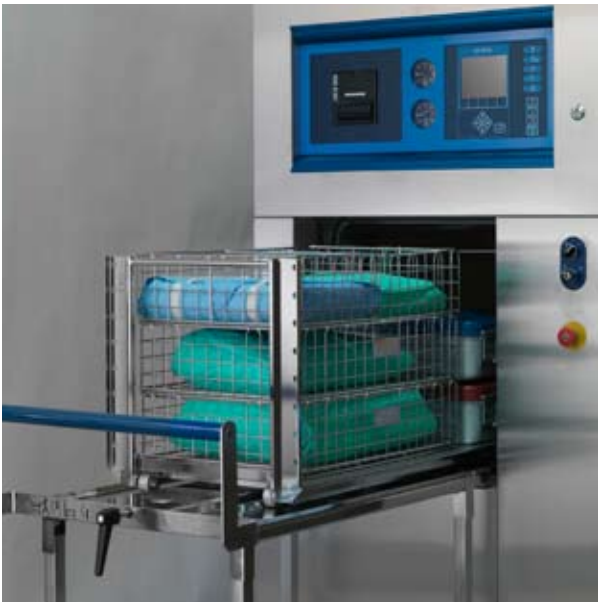
Manually Loading/Unloading of Shelf Rack. The shelf rack can be loaded with various load, e.g. containers and baskets. It can have shelves at 9 different levels.
