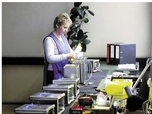
High voltage control and final inspection of all units.
