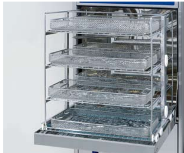
OP instrument wash cart (above) with 4 levels. All wash carts have removable shelves and spray arms.
