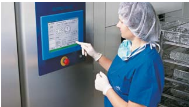
Getinge CM 320, a multi-chamber washer-disinfector , where the different phases of the process take place in different modules. Capacity can be adapted to changed requirements by adding modules. The wash racks are also adaptable with Getinge 8668 washer-disinfectors, so the different models can be combined.
